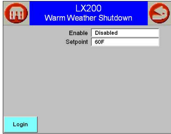
Figure 4-10 WWSD Configuration Screen
