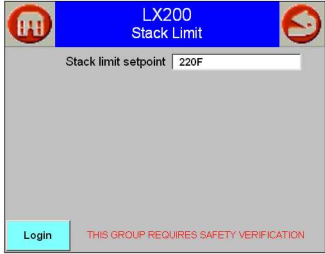
Figure 4-17 Stack Limit Screen
